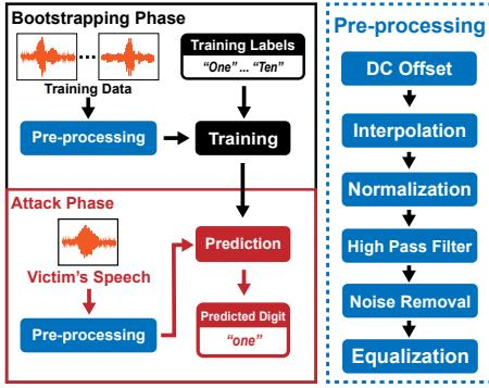
**Figure 2: Figure depicts the design overview of *LidarPhone*. The recovered audio signal from *LidarPhone* is pre-processed and used to train a model for digit, gender, or speaker identity inferences.**
