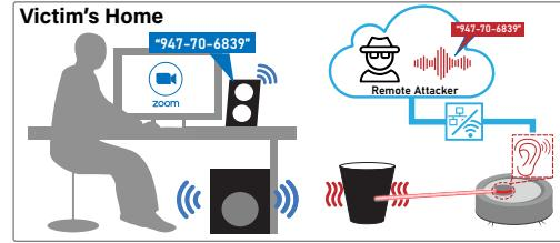
**Figure 1: An example of a *LidarPhone* attack. The adversary remotely exploits the lidar sensor on a victim’s robot vacuum cleaner to recover privacy sensitive information (e.g., credit card numbers) during a teleconferencing meeting.**
